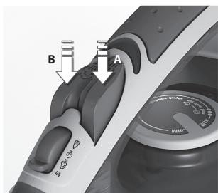
**4. Using the spray mist and steam jet function.** Ensure that water tank is at least 1/4 full. Use spray mist to pre-dampen fabrics by pressing spray button several times to release a fine mist (A). To use the steam jet function, ensure that tank is at least 1/2 full. Press steam jet button several times to prime pump (B).
