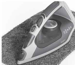
**3. Cleaning the soleplate.** Do not use scouring pads or harsh cleaners on the soleplate as these will damage the surface. To remove burnt residue, iron over a damp cloth while iron is still hot. To clean the Glissium™ soleplate (enamelled), simply wipe with soft damp cloth and wipe dry.
