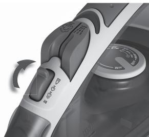
**2. Self-cleaning function.** Hold iron over a sink. Fill with water. Heat up iron. Move steam button to self-cleaning position, hold for 5 seconds to empty water from steam holes. Release button to stop self-cleaning function.
