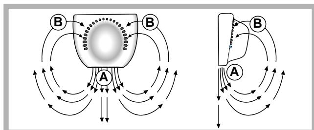
The A.I.R. System maintains a constant fridge temperature to keep food fresher for longer and will quickly restore the temperature to the correct level, even if the door is opened frequently: the blown air (A) is cooled when it comes into contact with the cold wall, whereas the hotter air (B) is sucked up (see diagram).
