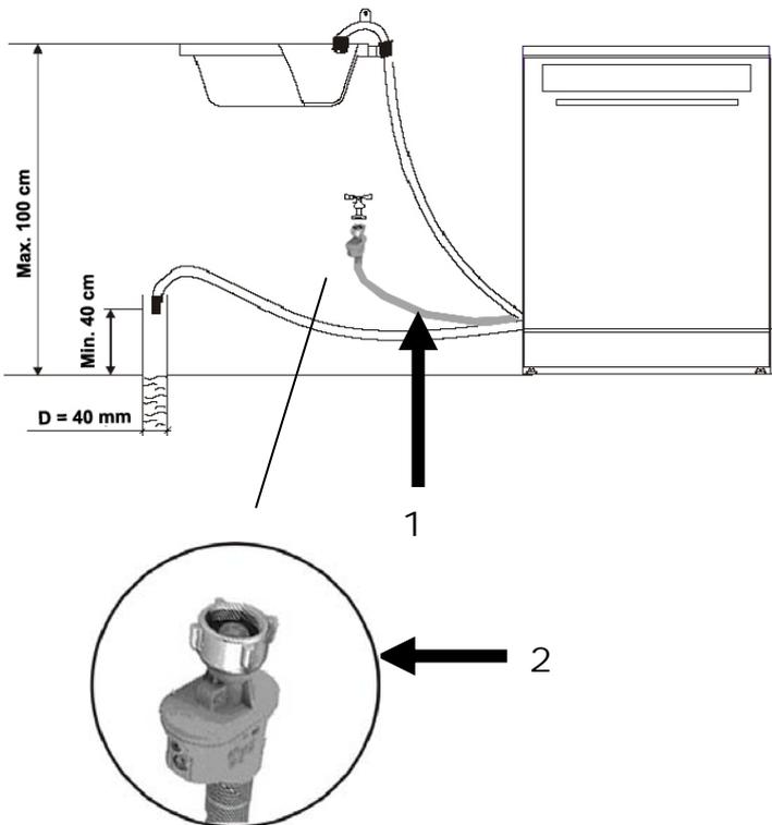
The inlet hose equipped with Aqua-Stop System 1 is provided with double walls. The Aqua-Stop System ensures blocking of water supply in case the inlet hose has broken as well as if the air gap between the hose itself and its corrugated shell is filled with water.
