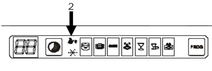
The salt container must be refilled when the salt warning light 2 comes on. Usually, the salt warning light is still on for a certain time after the salt container is refilled with salt and goes out as soon as the salt has dissolved completely.
