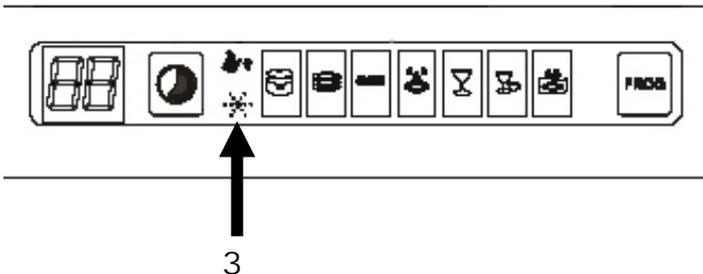
The rinse aid should be added, when the Rinse aid warning light 3 on the control panel goes on.
