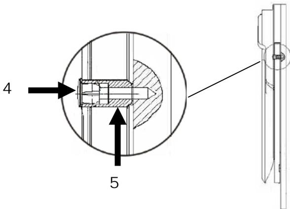
After that it is necessary to fix the panel on a door of a dishwasher by screws from the inside of the door through corresponding holes 3.
