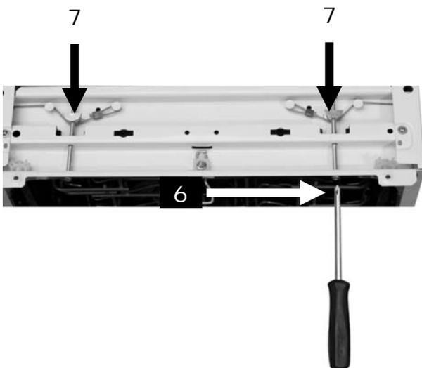
The door springs are set at the factory to the proper tension for the outer door. If aesthetic wooden panel are installed, you will have to adjust the door spring tension. Rotate the adjusting screw 6 to drive the adjuster 7 to strain or relax the steel cable.
