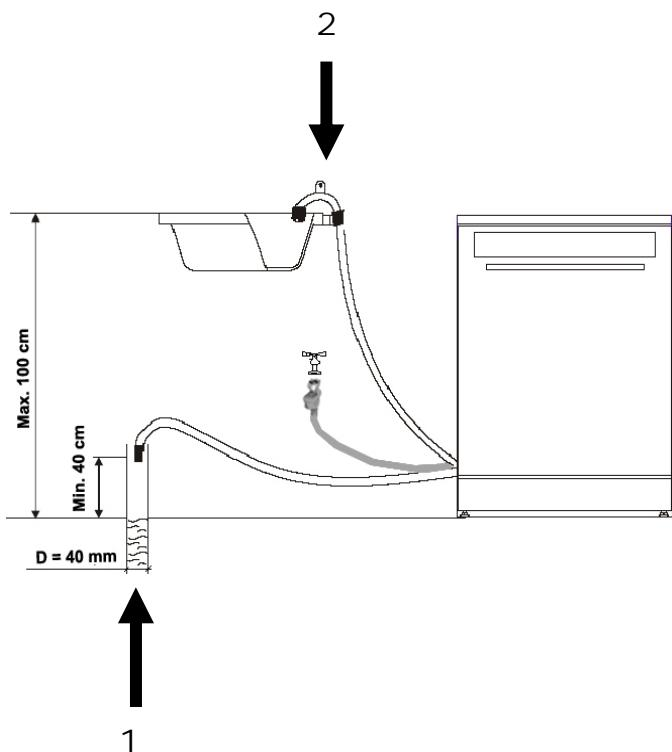
Use the special plastic hose support which is delivered with the appliance.
