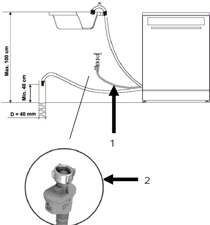
The inlet hose equipped with Aqua-Stop System 1 is provided with double walls.
