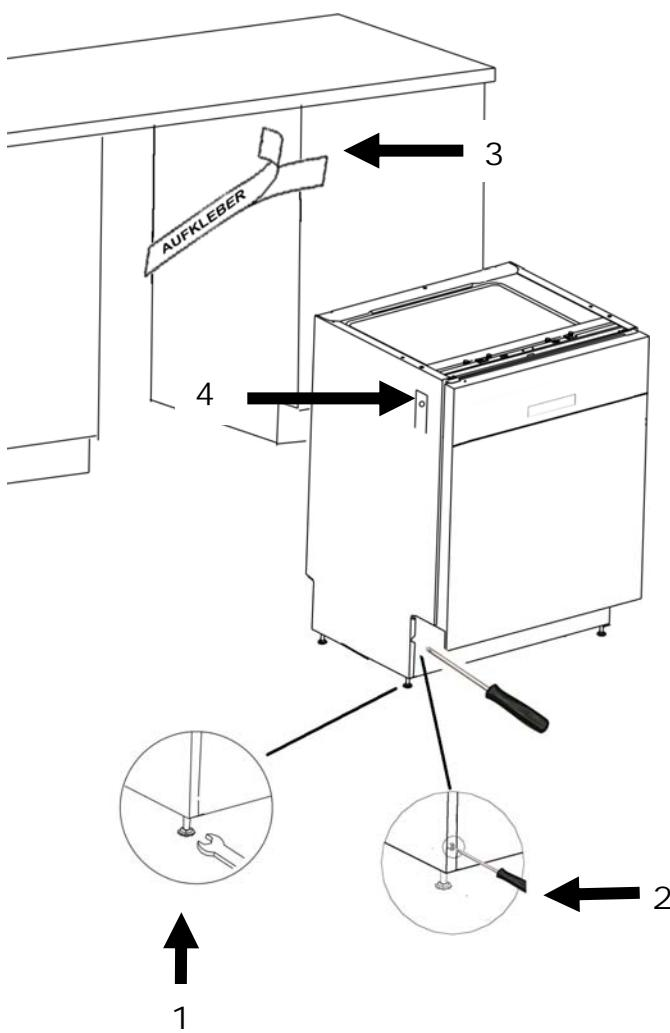
Once the appliance is positioned, level the dishwasher by adjusting the feet 1 and 2 (screw in or out). The inclination angle must not exceed more than 2°.
