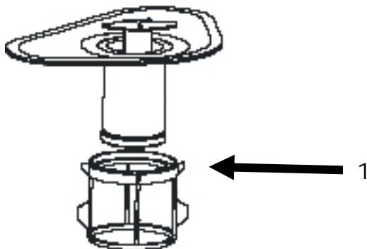
To clean the coarse filter and the fine filter, use a cleaning brush.
