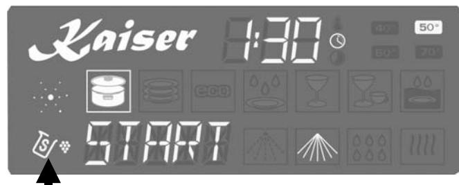
The salt container must be refilled when the salt warning light 2 comes on. Usually, the salt warning light is still on for a certain time after the salt container is refilled with salt and goes out as soon as the salt has dissolved completely.
