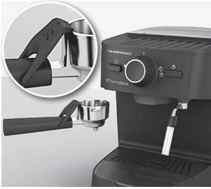
**7. After brewing**, remove the filter holder. Twist it to the left and take it out of the retainer. Fold finger protector forwards and remove used coffee grounds from the filter. Then take it out of the holder and clean it with water. Dry with a cloth before putting it back into the filter box.
