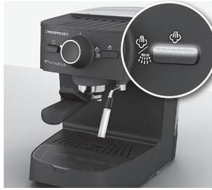
**1. Steam can be used** to froth milk or to heat liquids. Push the steam button and wait for the steam temperature indicator light to stop flashing and go to constant light. Immerse the steam nozzle in a heatproof container with milk.
