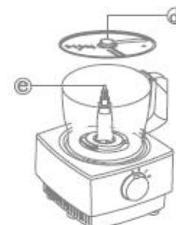
1). Fit the drive shaft and bowl onto the power unit.
