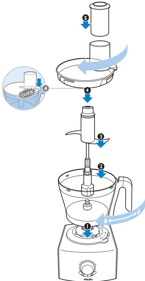
**EN** | Assembly/disassembly
