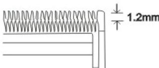
If the blades were removed for cleaning or replacement, they must be leveled. Align the blades on the plane and tighten the fixing screws.
