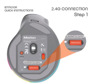
Take out the usb receiver on the bottom of the mouse
