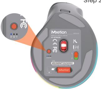
Short press the mode switch button at the bottom of the mouse, the \$1 blue light flashes slowly
