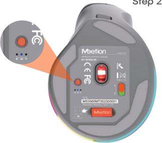
Short press the mode switch button at the bottom of the mouse, the 32 blue light flashes slowly
