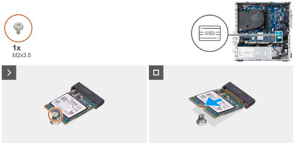
Figure 22. Removing the M.2 2230 solid state drive
