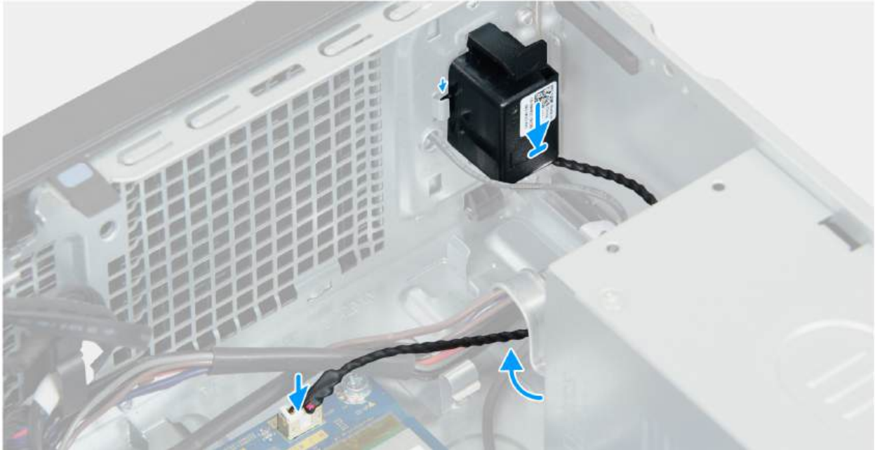
Figure 19. Installing the internal speaker
