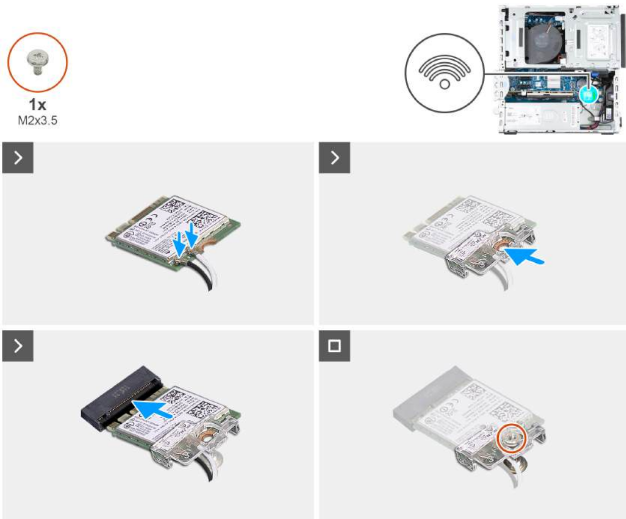
Figure 30. Installing the wireless card
