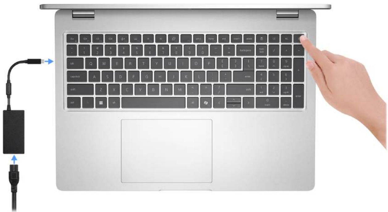
Figure 11. Connect the power adapter and press the power button
