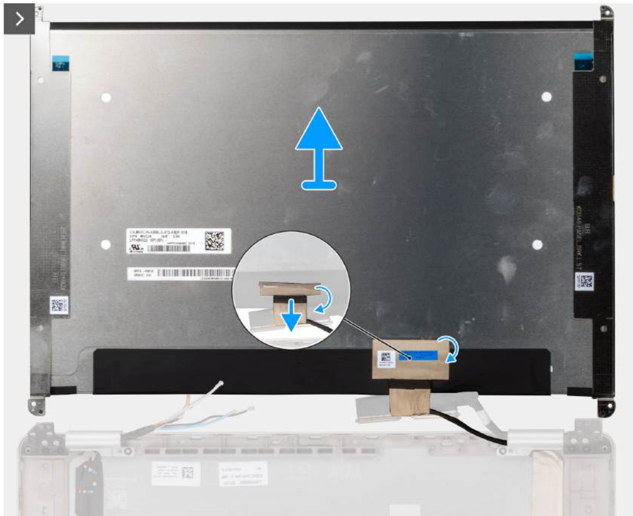
Figure 73. Removing the display panel
