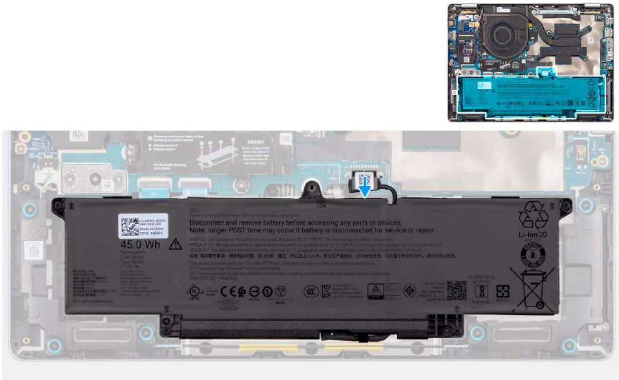
Figure 19. Disconnecting the battery cable
