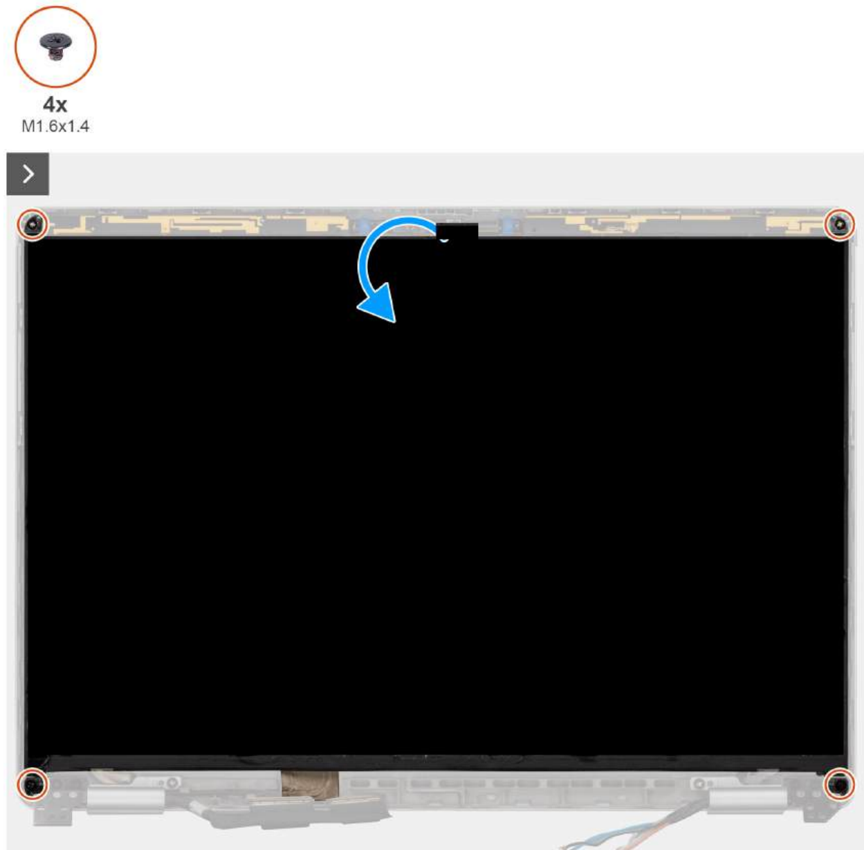
Figure 72. Removing the display panel
