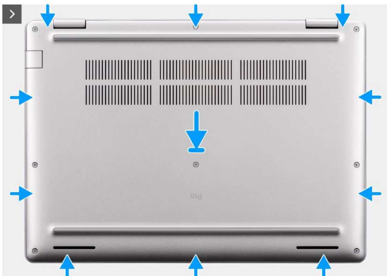
Figure 21. Installing the base cover
