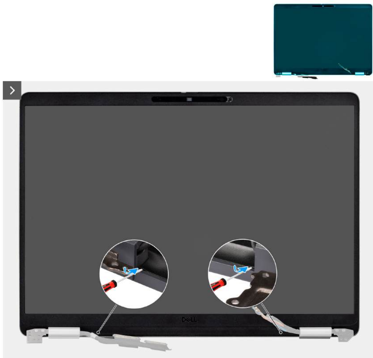
Figure 65. Prying the plastic bezel
