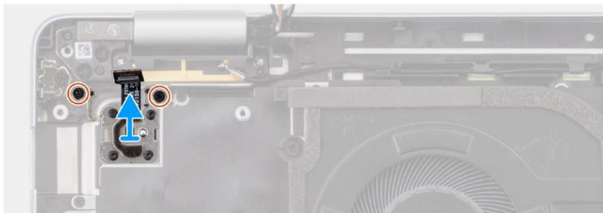
Figure 59. Remove the power button with optional fingerprint reader
