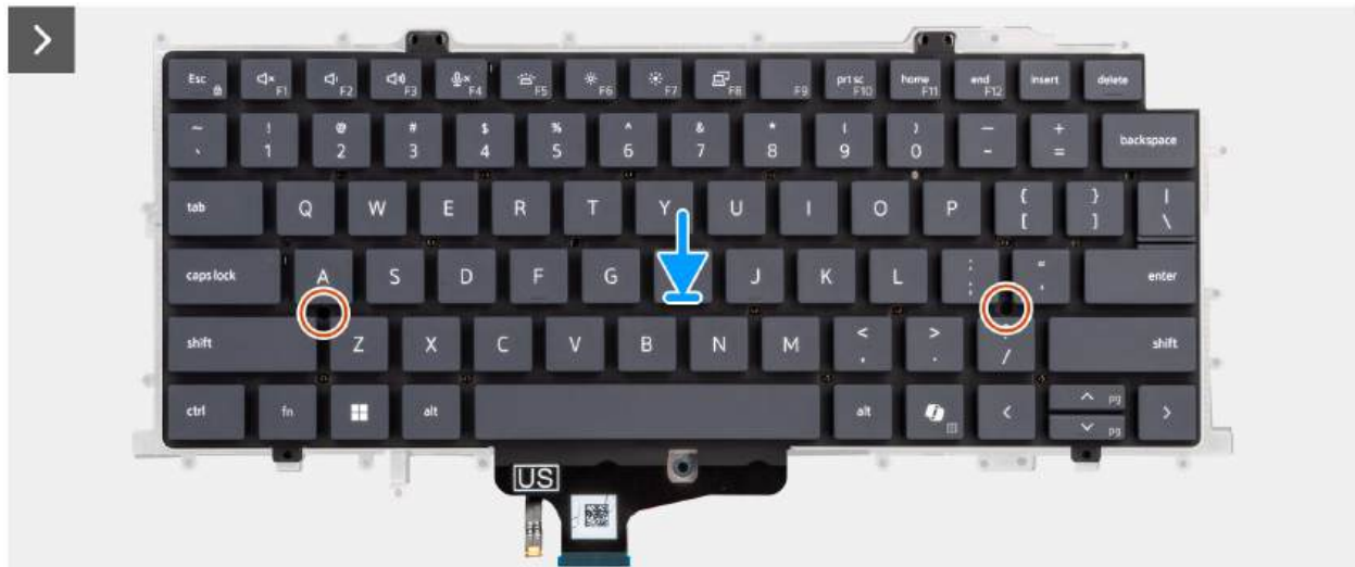
Figure 99. Installing the keyboard
