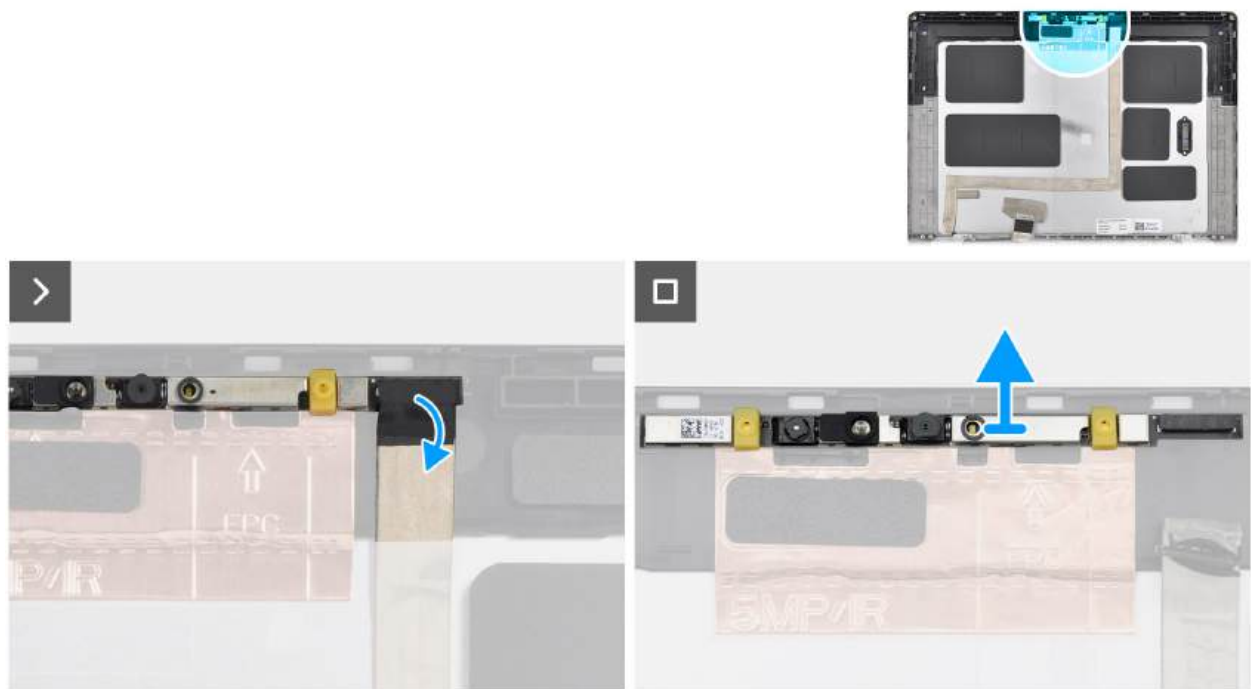
Figure 79. Removing the IR camera
