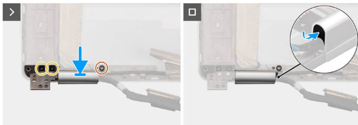
Figure 88. Installing the display cable for RGB/IR camera
