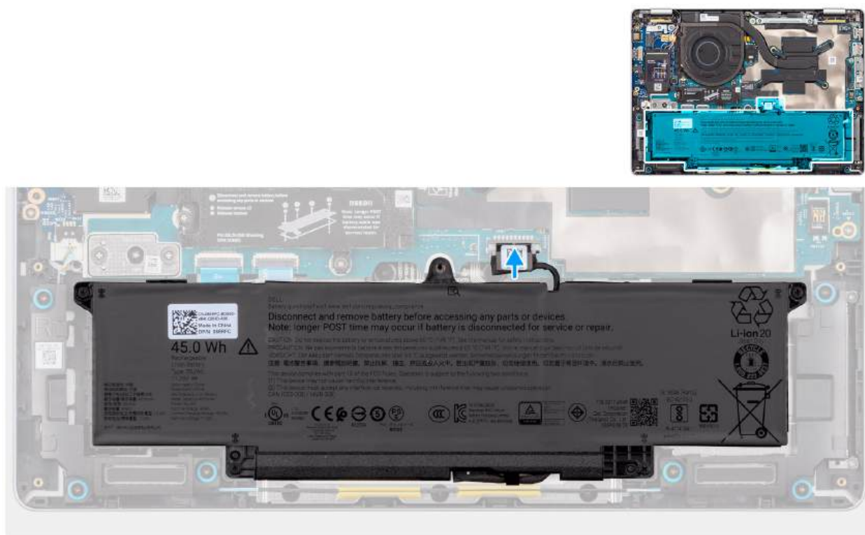
Figure 20. Connecting the battery cable
