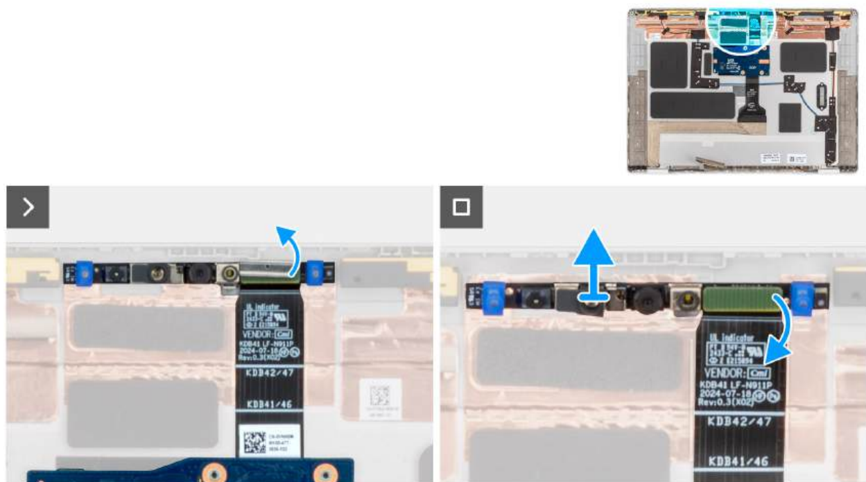
Figure 83. Removing the MIPI camera
