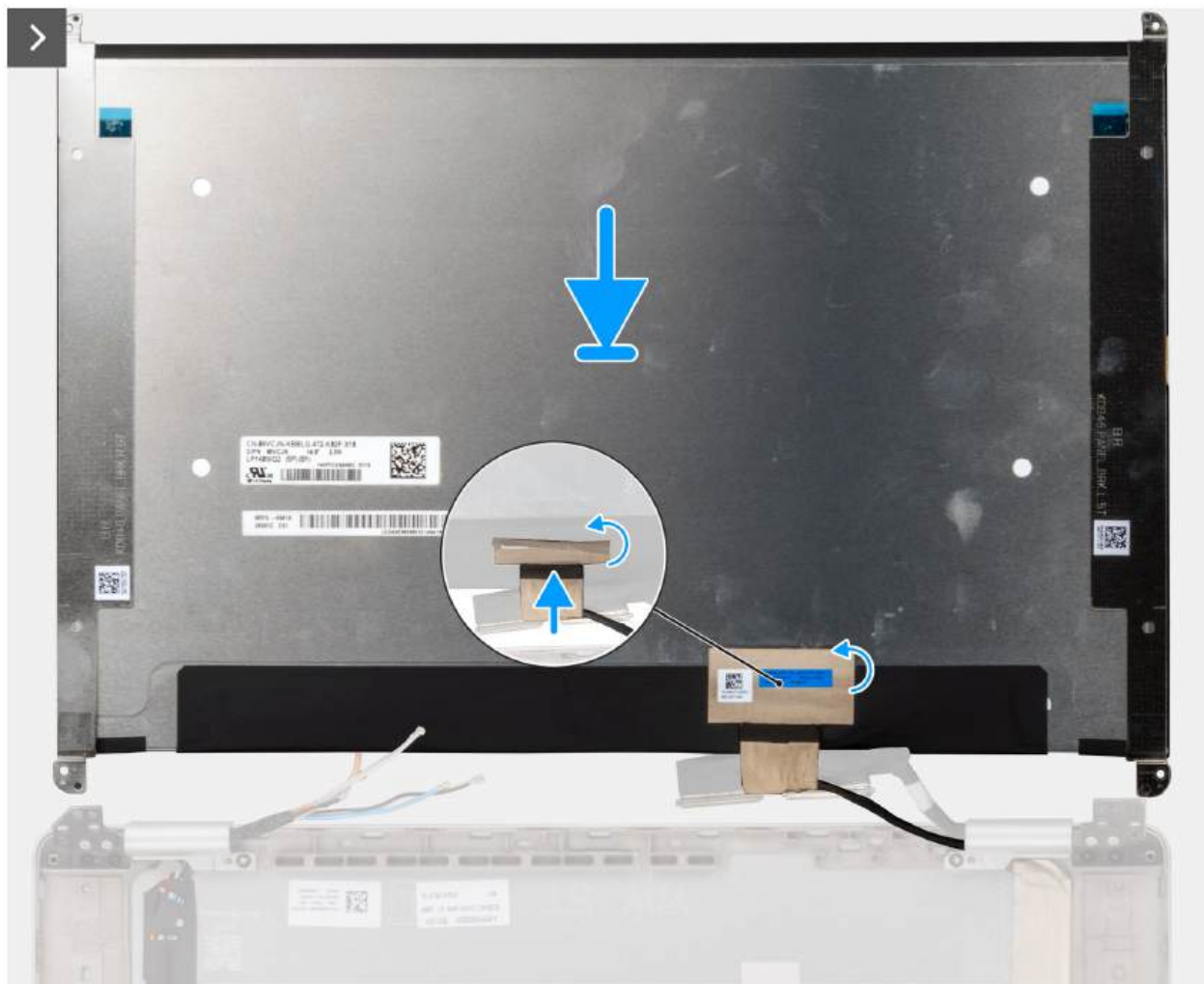
Figure 75. Installing the display panel
