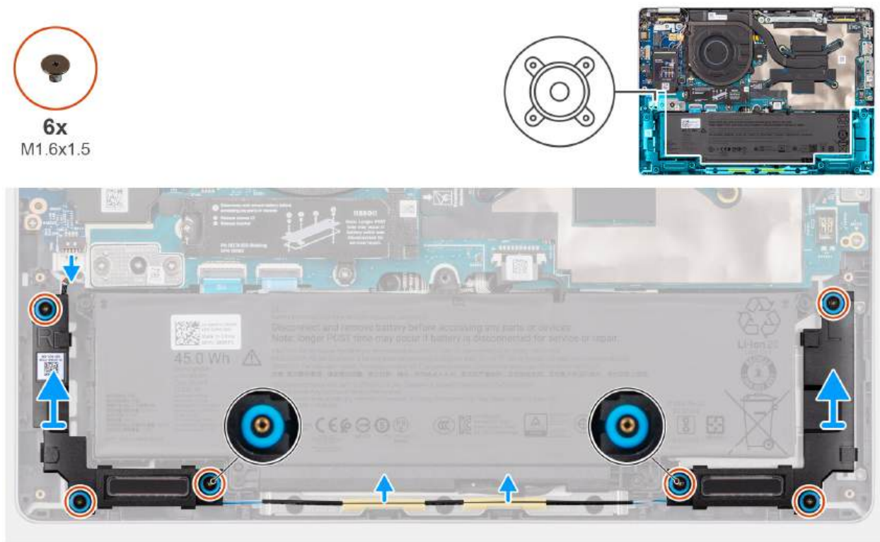
Figure 35. Removing the speakers
