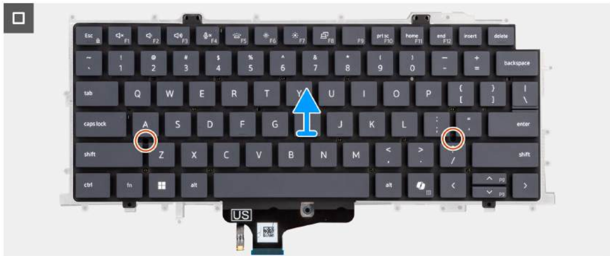
Figure 98. Removing the keyboard
