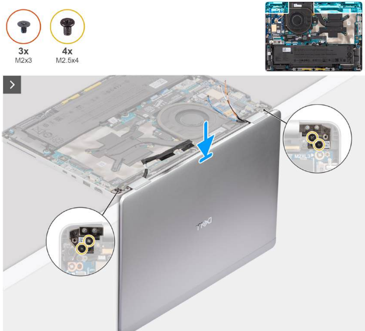
Figure 63. Aligning the display assembly with the palm-rest assembly
