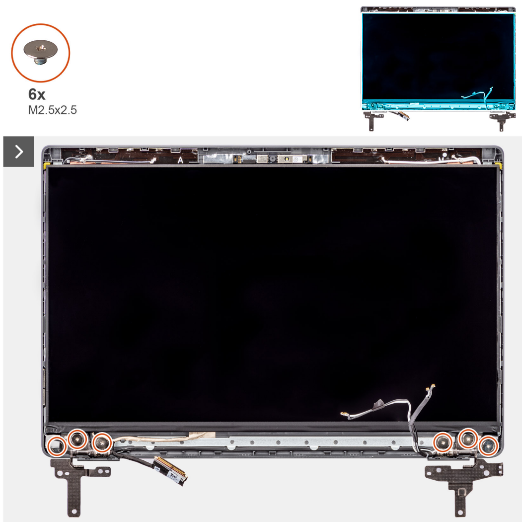
Figure 54. Removing the display panel
