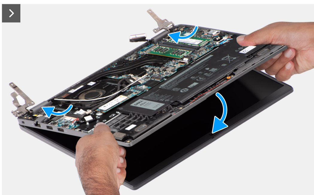
Figure 49. Removing the display assembly
