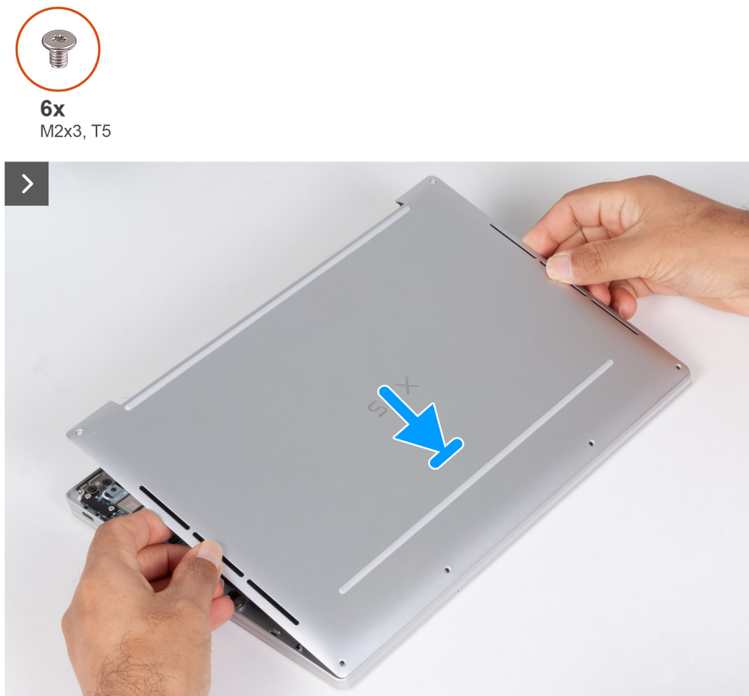
Figure 12. Installing the base cover
