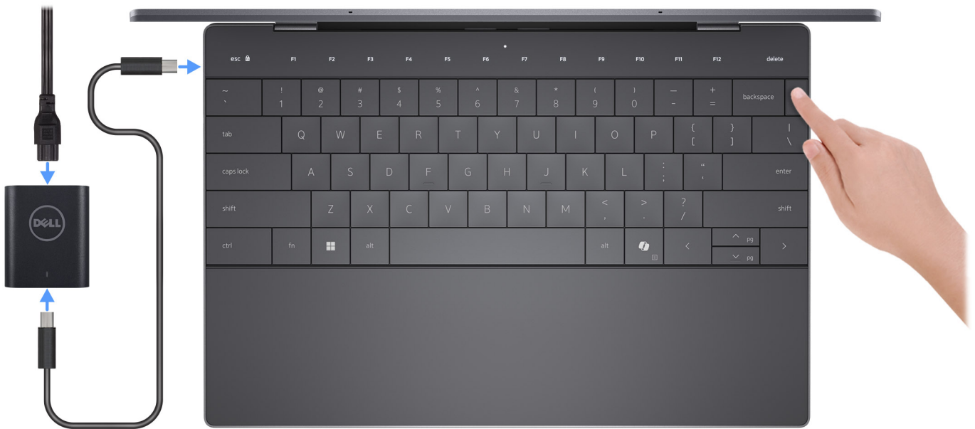
Figure 7. Connect the power adapter and press the power button.
