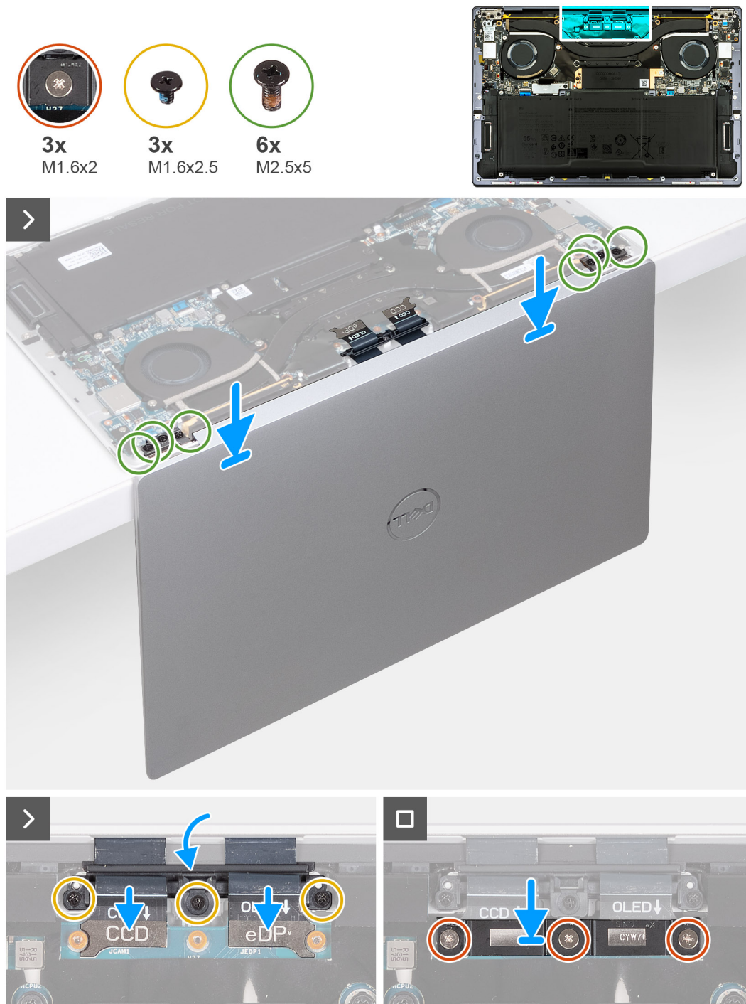
Figure 33. Installing the display assembly
