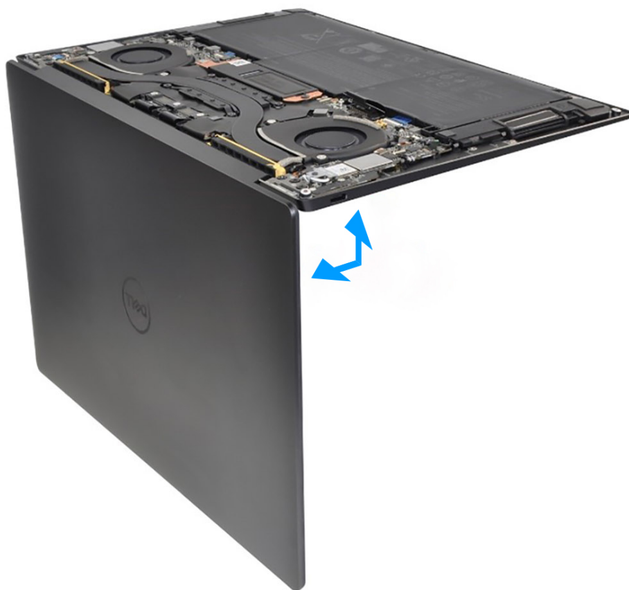
Figure 35. Opening the display assembly to a 90-degree angle
