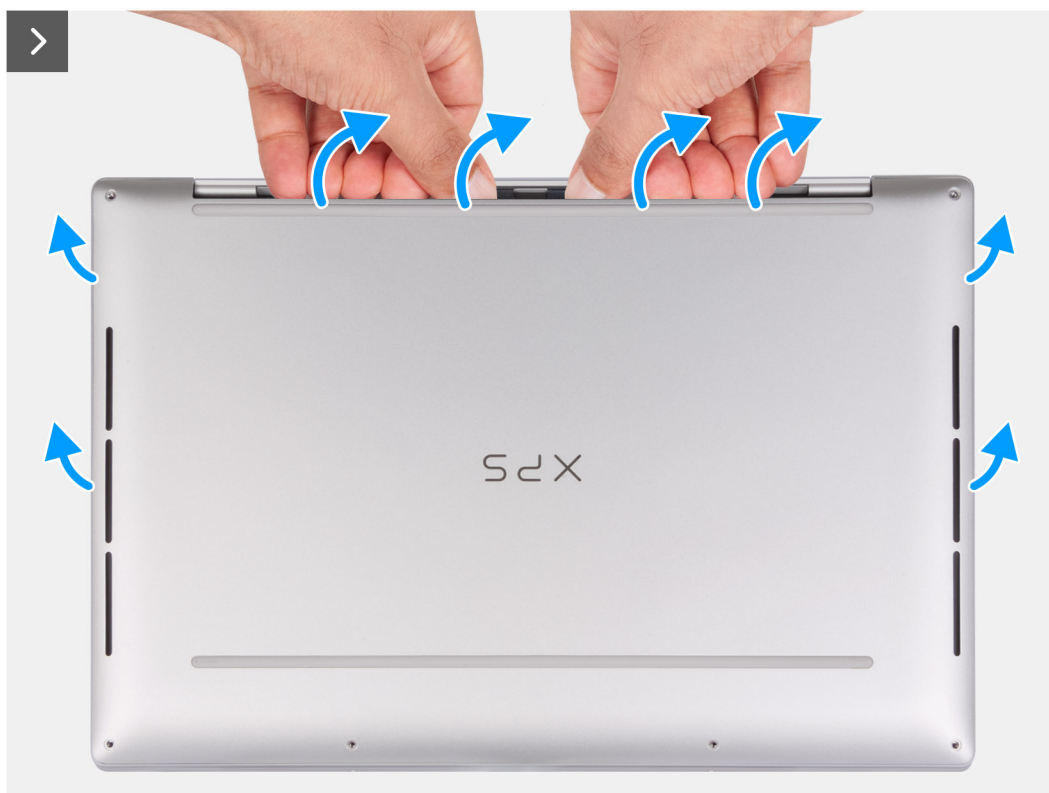
Figure 10. Removing the base cover
