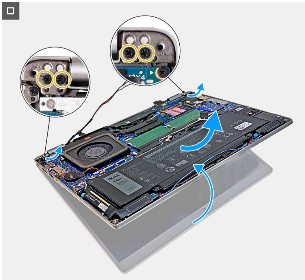
Figure 46. Removing the display assembly - For computers shipped with 5G card
