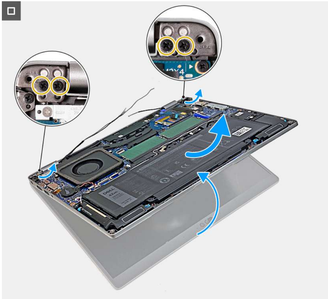
Figure 44. Removing the display assembly - For computers shipped with 4G card
