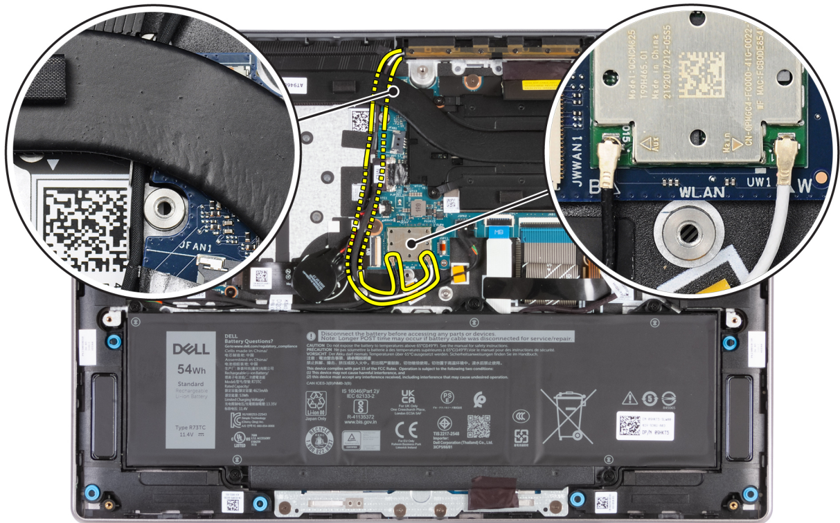
Figure 71. Installing WLAN-antenna cables
