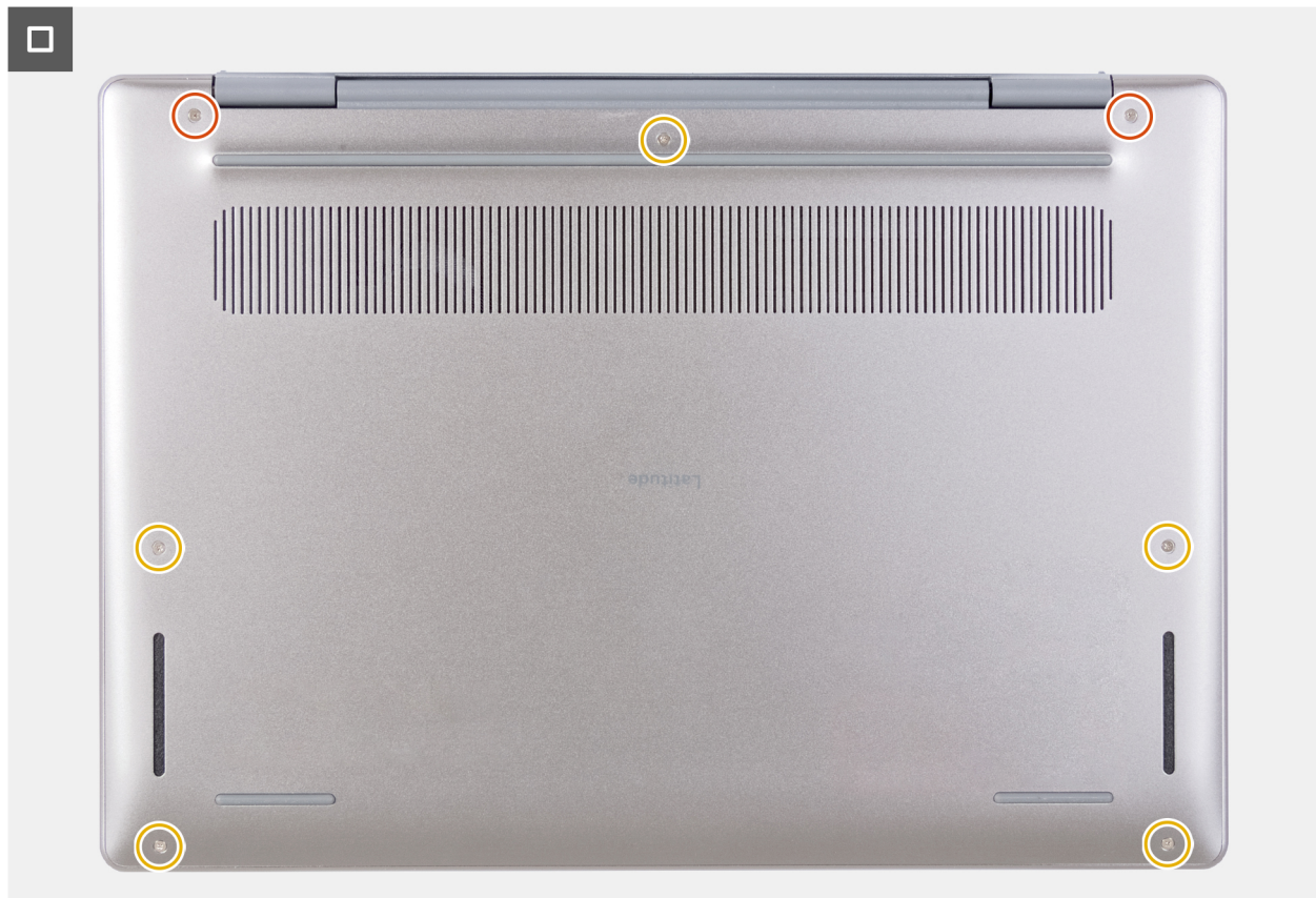
Figure 20. Tightening and replacing the screws
