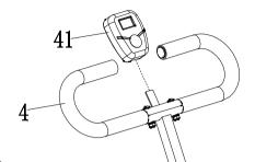
Insert the Monitor(#41) onto the tab of the Handle Bar(#4).
