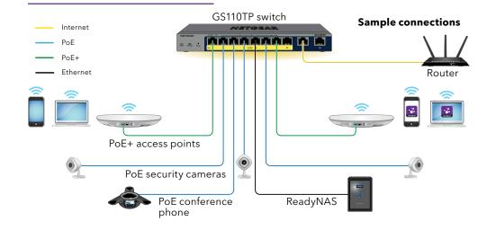
This switch is designed for indoor use only. If you want to connect to a device located outdoors, the outdoor device must be properly grounded and surge protected, and you must install an Ethernet surge protector inline between the switch and the outdoor device. Failure to do so can damage the switch.
