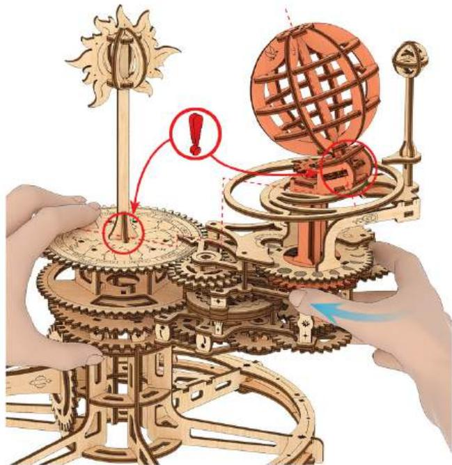
**ENG** Rotate the Earth's drive gear clockwise until there is an imaginary straight line from the back of the Earth through the "Earth-Moon" pointer to the center of the season sector.
