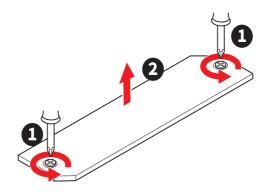
3. If you install 2260 SSD, use the included EZ M.2 Clip II Remover. Place the included EZ M.2 Clip II in the slot, use the remover to screw it in by turning it clockwise, and secure it. Skip this step if you install 2280 SSD.
