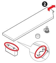
3. If you install 2260 SSD, install the supplied M.2 standoff in 2260 hole. Skip this step if you install 2280 SSD.
