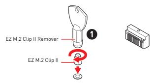
2. Insert your M.2 SSD into the M.2 slot at a 30-degree angle. Use the EZ M.2 Clip II, which automatically locks and secures the SSD.
