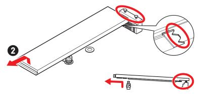
3. If you install 2260 SSD, use the included **EZ M.2 Clip II Remover**. Place the included **EZ M.2 Clip II** in the slot, use the remover to screw it in by turning clockwise, and secure it. Skip this step if you install 2280 SSD.
