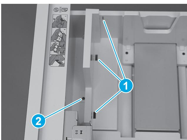
**EN** Align the left front guide to the LTR slots in the bottom and side of the tray (callout 1), and then reinstall the screw (callout 2).
