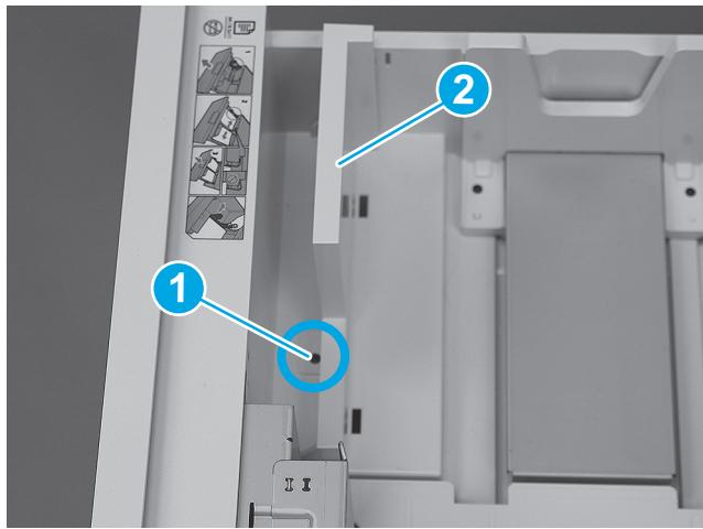
**EN** Remove one screw (callout 1), and then remove the left front guide (callout 2).
