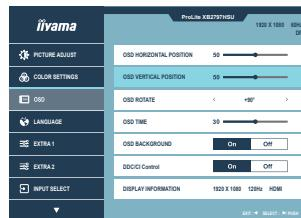
Press or tilt the Joystick [Center] and finally tilt it [ $\uparrow$ ] to close the On Screen Display feature. All changes are saved in the memory.
