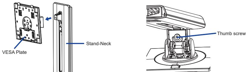
② Install the Stand-Base to the Stand-Neck and then tighten the 'thumb screw' with the provided screwdriver to secure them.
