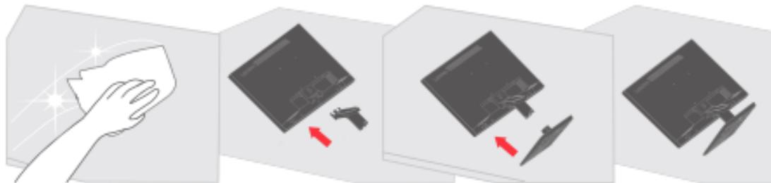
1. Place the display screen down on a soft flat surface.
