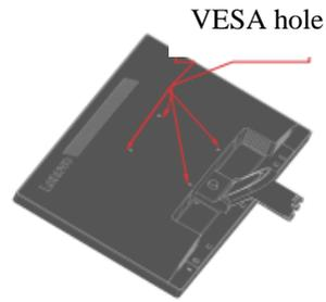
Step 5: Mount the LCD to the wall following the instructions for the wall mount. Only the lightest weight/weight-bearing wall mount from the UL list should be used: 8kg
