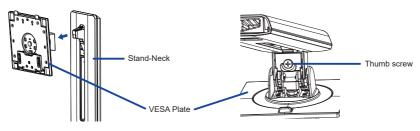
② Install the Stand-Neck to the Stand-Base and then tighten the 'thumb screw' to secure them.
