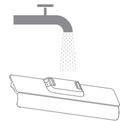
2. The brush cover can be rinsed with clean water or wiped completely before reuse.
