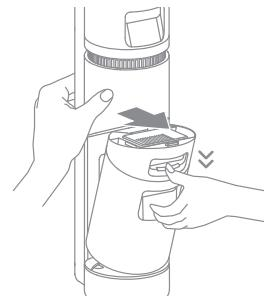
2. Take out the filter from the Used Water Tank cover. Remove the tank cover and pour out the used water.
