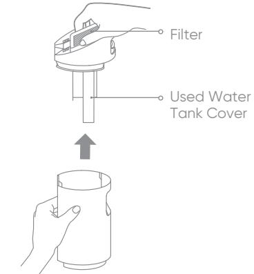
3. Rinse the Used Water Tank and the tank cover with clean water. Clean the tank by the provided cleaning brush.
