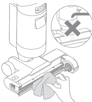
**Warning:** To reduce the risk of electric shock or injury, do not rinse the roller brush assembly with water!
