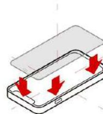
Attach the film, make sure that it is centered, and the cutouts do not cover the speakers and cameras
