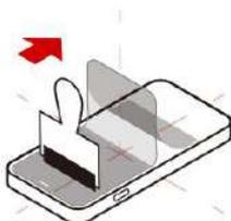
Holding one half, remove installation cover starting from the center
